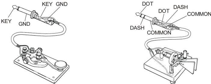
For straight-key operation, only the tip and shaft connections are used.
