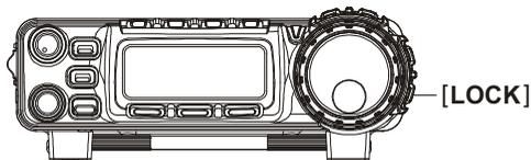
In the transceiver's default configuration, pressing the **[LOCK]** button disables just the **DIAL**, while the other keys and switches are unaffected. To lock out the remainder of the controls and the **SELECT** knob, use Menu Mode No-054 **[LOCK MODE]**:
