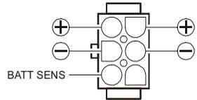
lead connects to the Negative (-) side of the power source. This Jack also provides an Transmit Power Control terminal. If you connect pin-3 (BATT SENS) of the DC power jack to the ground, the **FT-857D** automatically switches to 20 Watts (430 MHz: 10 Watts) of output power.
