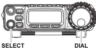
The synthesizer steps for the **SELECT** knob may be adjusted independently by mode. Use Menu Mode No-006 [AM STEP] for AM, No-052 [FM STEP] for FM, and No-082 [SSB STEP] for SSB/CW/DIG. See pages 97, 105, and 110 for details.
