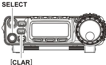
If you wish to make a more permanent shift in the receiver's IF passband, use Menu Mode No-015 [CAR LSB R] (for LSB mode) or No-017 [CAR USB R] (for USB mode). This allows you to set up a higher or lower listening pitch, if you prefer such as compared to the default passband response. See page 99.
