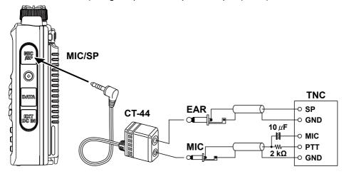
After connecting the TNC to the transceiver, set the output signal level to the TNC by adjusting the sound volume level of your transceiver.
