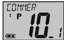
4. Press the [PRESET] key to program the current channel into the Preset channel bank.
