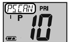
ter each Preset channel. The “PSCAN” notation will appear at the upper left corner of the display during scanning.
