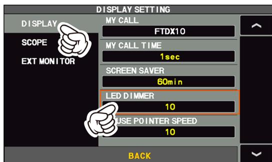
4. Rotate the [FUNC] knob, or touch "<" or ">" on either side of the value to adjust the brightness.
