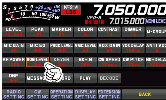
3. Rotate the [FUNC] knob to adjust the Monitor level.
