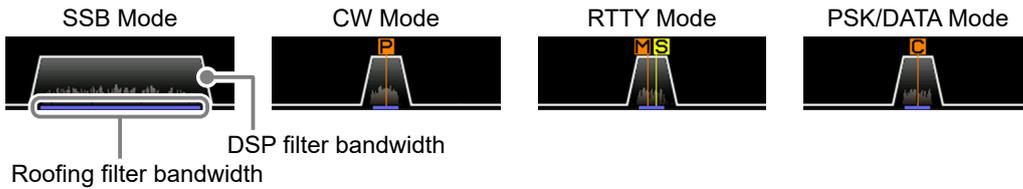
Touch the filter display to reveal and check the setting value of the last used function from SHIFT, WIDTH, NOTCH, CONTOUR, and APF. The setting may be changed by turning the knob of the active function.
