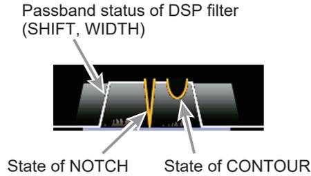
The current roofing filter bandwidth is displayed as a blue line below the filter function display.
