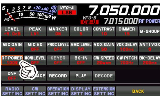
3. Rotate the [FUNC] knob to adjust the RF power.
