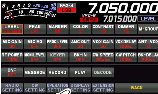
3. Touch [DISPLAY] → [SCREEN SAVER] or rotate the [FUNC] knob to select an item and press the [FUNC] knob.
