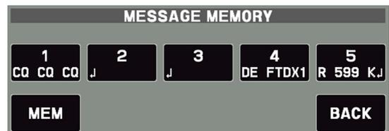
4. Touch [1] through [5] key, depending on which PSK Text Memory Register message you wish to transmit. The programmed message will be transmitted on the air.
