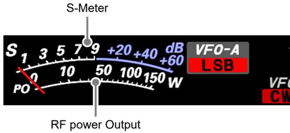
When the meter display screen is touched, the transmit meter selection screen is shown (the default setting is “PO”).
