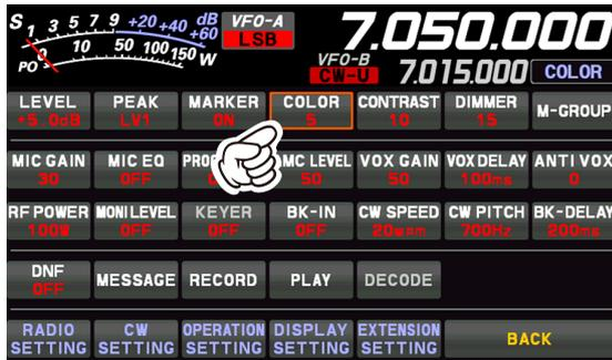
The Display Color selection screen will disappear automatically after about 3 seconds.
