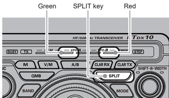
During Split operation, the VFO-A register will be used for reception, while the VFO-B register will be used for transmission. If you press the [SPLIT] key once more, Split operation will be cancelled.
