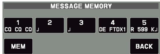
4. Touch [1] through [5] key, depending on which RTTY Text Memory Register message is to be transmitted. The programmed message will be transmitted on the air.
