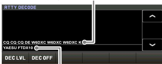
Displays text entered into the RTTY sending memory.
