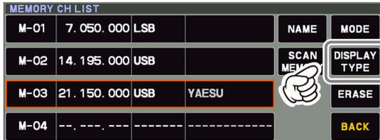
4. Rotate the [FUNC] knob to select the desired display type.
