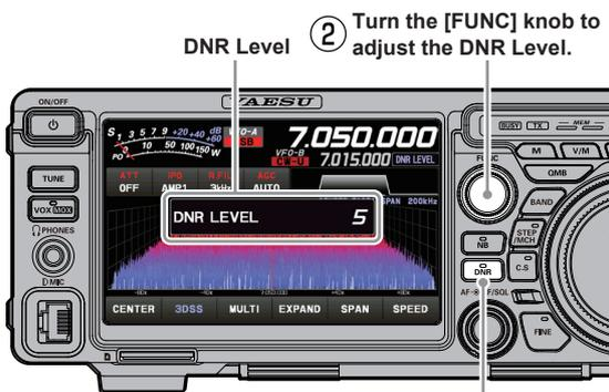
① Press and hold the [DNR] key to display the DNR level.
