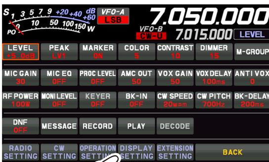
3. Touch [DISPLAY] → [LED DIMMER] or rotate the [FUNC] knob to select an item and press the [FUNC] knob.
