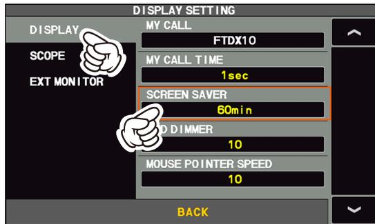
4. Rotate the [FUNC] knob, or touch “<” or “>” on either side of the value to select the time until the screen saver is employed (default setting is 60 min).
