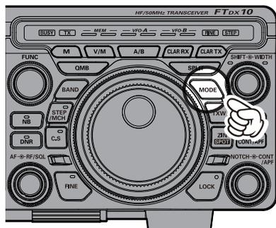
2. The operation MODE selection screen appears on the display, then touch [PRESET], or rotate the MPVD ring to select [PRESET].
