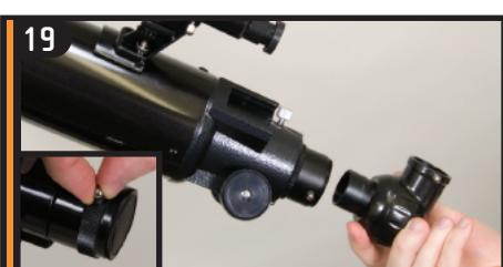
Loosen the set screws on the focuser so that they do not obstruct the inner diameter of the focuser. Insert diagonal into the focuser and tighten the set screw.
