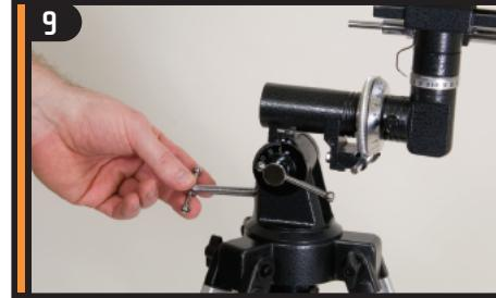
Thread the latitude adjustment screw into the equatorial mount until it is touching the inside of the mount.
