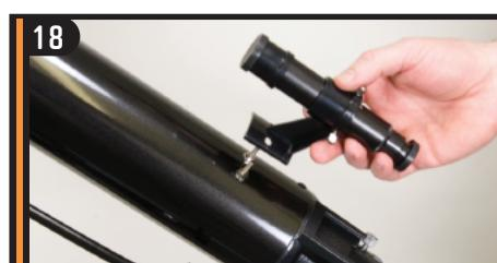
Orient the finderscope so that the glass window is facing towards the front of the tube. Place finderscope over the holes on the tube and replace the knurled nuts to secure.
