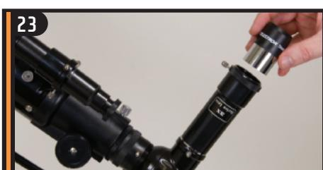
Place the eyepiece into the barlow and tighten the set screw to secure in place.
