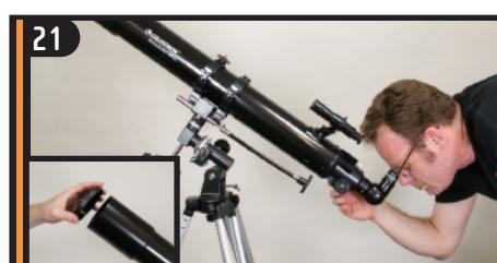
Remove the lens cap from the front of the telescope. To observe, look through the eyepiece as shown above.
