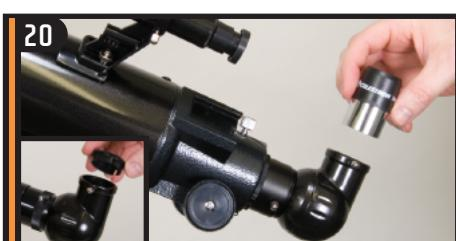
Remove cap and insert the 20mm eyepiece into the diagonal and tighten the set screw.
