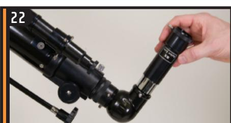
For additional magnification, you can use the included 3x barlow. Place the barlow in the focuser in place of the eyepiece – remove the cap from the barlow.
