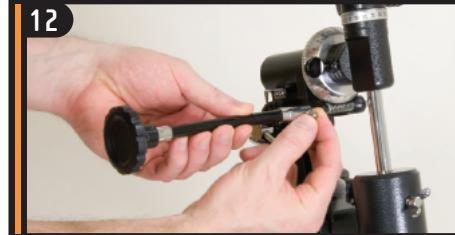
Slide the chrome end of the slow motion control cable onto equatorial mount gear shaft and tighten screw to secure in place.
