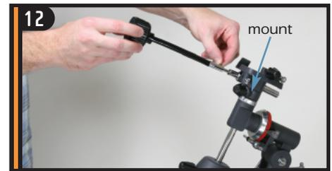
Slide the chrome end of the slow motion control cable onto declination axis gear shaft.
