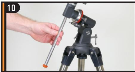
Tighten the threaded end of the counterweight bar into the Dec axis of the equatorial mount.
