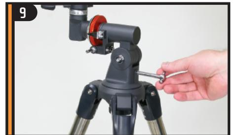
Thread the latitude adjustment screw into the equatorial mount until the screw is touching the inside of the mount.
