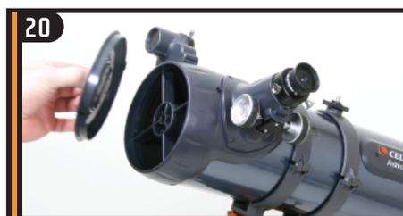
Remove the lens cap from the front of the telescope before you begin observing.
