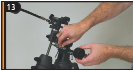
The other cable attaches to the R.A. axis gear shaft.
