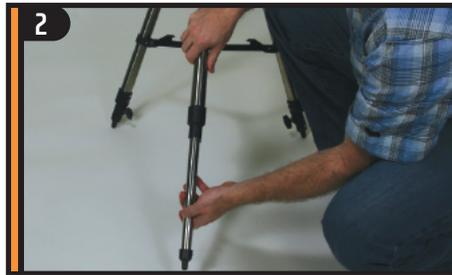
To set up the tripod, spread the legs outward until they are fully extended. Extend the center portion of each of the three tripod legs down 6-12".
