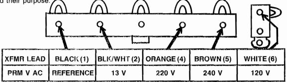
This chart shows the color code of the transformer leads and their purpose. The number in parenthesis indicates the number of the terminal lug that the transformer lead is connected to. The number three (3) lug is not used to change the filament or blower wiring. Do not add or remove any wires from the number three (3) lug. Refer to the drawing above. Use the lug numbers above when referring to both of the Filament connection chart and the Blower connection chart below.
