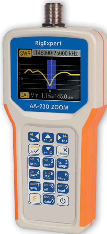
**RigExpert AA-230 ZOOM** is a new powerful antenna analyzer designed for testing, checking, tuning or repairing antennas and antenna feedlines.
